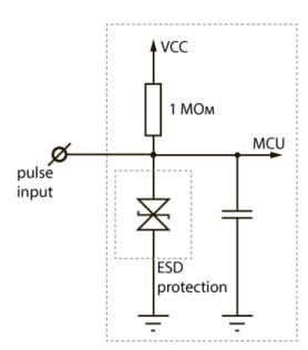
De-bouncing logics with 5 msec time constant is integrated in the pulse counter. The pulse counting is carried out for frequencies up to 200 Hz.
